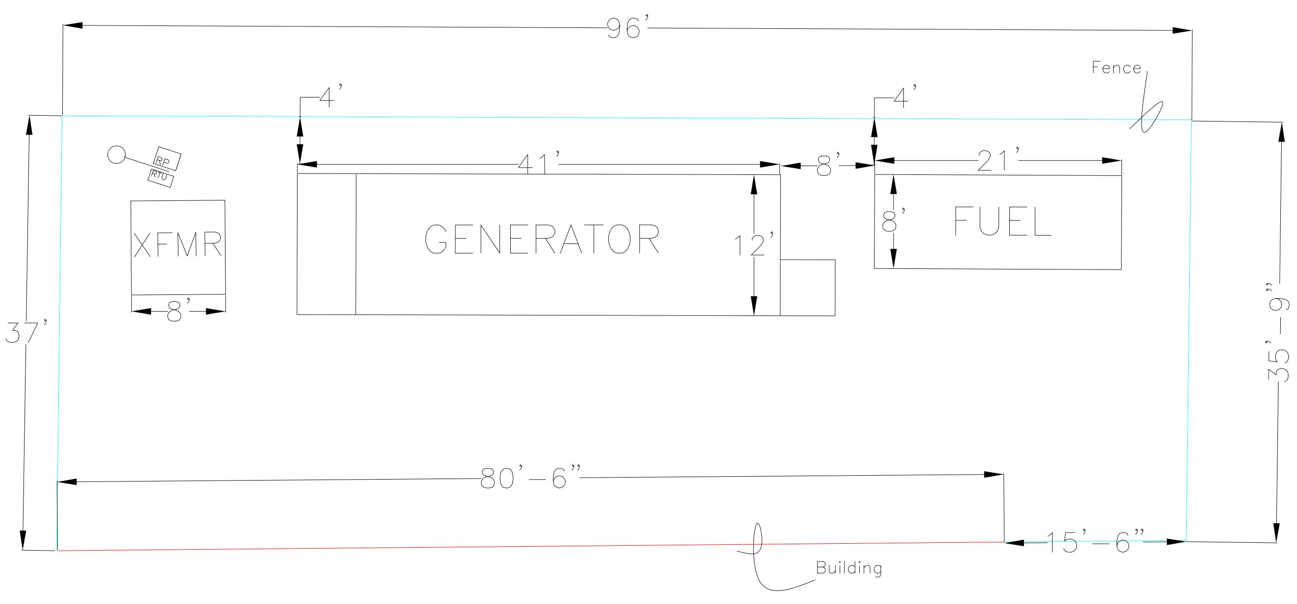
Note: Transformer Pad (XFMR) to remain in place with existing transformer. Fuel tank pad to be removed. Generator pad to be removed if necessary. New Generator to occupy same footprint as existing generator and fuel tank.
